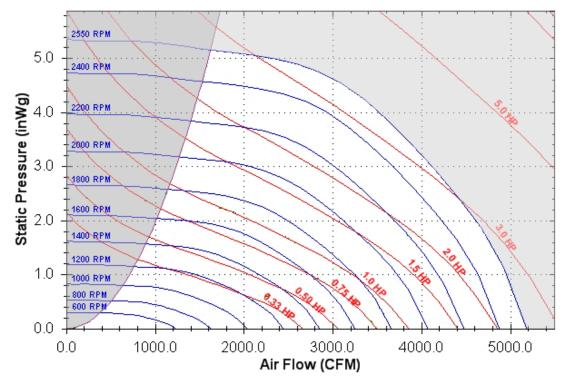
Figure 19: Fan Curve – 22 inch Fan
