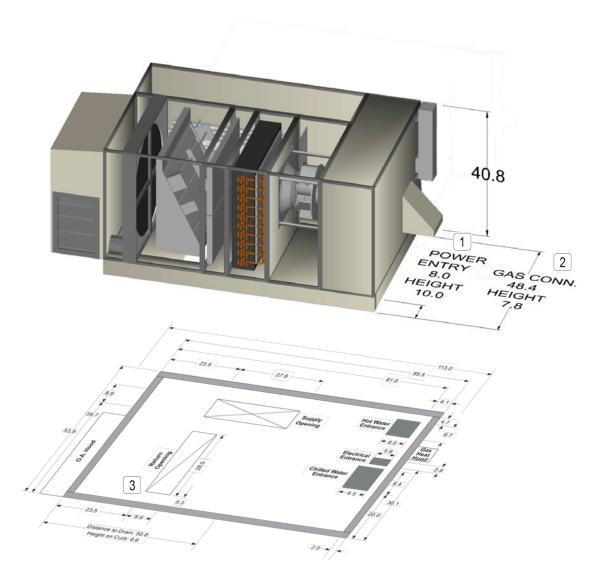
**NOTE:** 1. Recommended location for field cut side power connection
