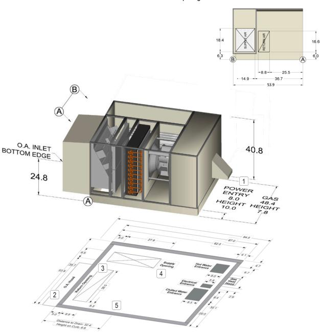
Detail: A-B Optional Horizontal Supply and Return Air Openings
