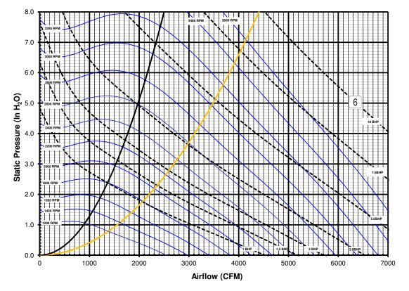
Figure 21: Fan Curve – DDPL-20 – Size 15–21
