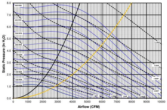
Figure 22: Fan Curve – DDPL-24 – Size 15–21
